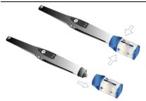
To remove the wireless pack, press the buttons on both sides of the pack and pull down to remove it from the camera. Be careful and gentle in order to preserve your wireless pack in working order.
